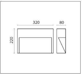
MODULES LED 3000K 230V 1650Im CRI 80 Rated luminaire luminous flux: 304Im Rated input power: 18W Luminaire efficacy: 17Im/W Electronic ballast 220÷240V 50/60Hz
