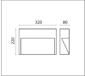
MODULES LED 3000K 230V 1650lm CRI 80 Rated luminaire luminous flux: 304lm Rated input power: 18W Luminaire efficacy: 17lm/W Electronic ballast 220÷240V 50/60Hz
