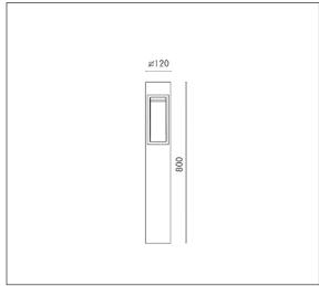
4 MODULES LED 3200K 230V 777Im 8.4W CRI 80 Rated luminaire luminous flux: 131Im
