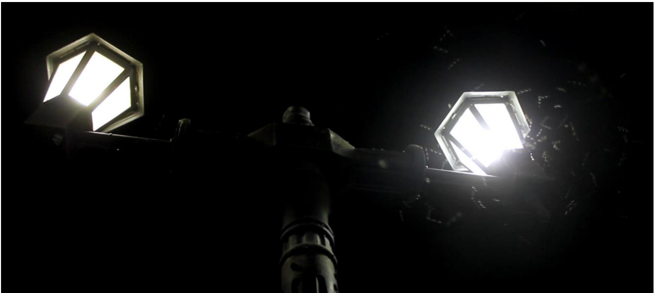
Fig. A7: These luminaires in Kalavrita show the influence of artificial light: left a warm white lamp with low blue content and nearly no insect activity. Right a cold white lamp with high blue content and many insects flying around (screen-shot from a video)
